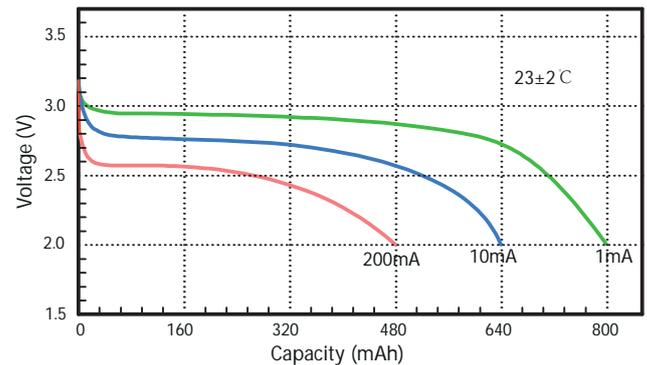
2. Voltage plateau versus Current and Temperature
